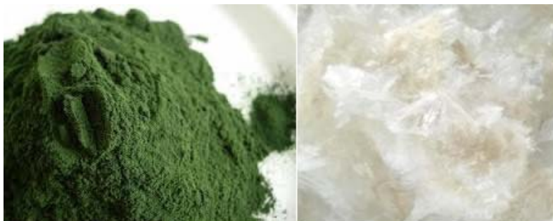
Fig. 1. Raw material (left) and solid extract (right): from commercially available dry Spirulina powder a polysaccharide extract was obtained and the effects of its aqueous solution was tested on paper in order to record its effects.
